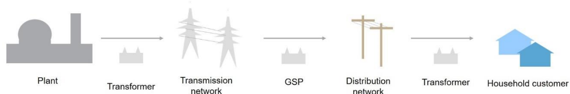
Figure 2: Overview of where losses can occur during electricity delivery to the user
